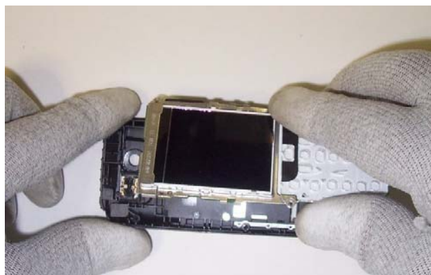
6) Lift and remove Engine Module Assembly
