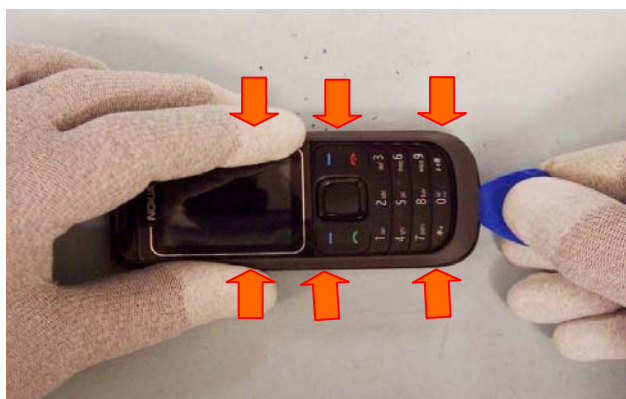
3) Insert SRT-6 from bottom and slide along sides to release 3 tabs one side and then 3 tabs another side.
