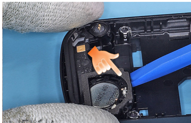
14) Use the SS-93 to remove the Antenna Module. Always start from the shown position.
