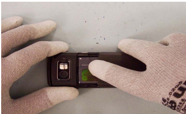
1) Unlock and remove the BATTERY COVER.
