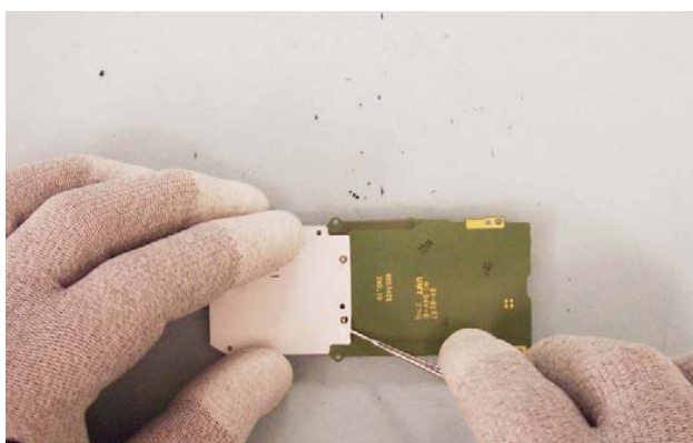
17) Use Pick to lift the Dome Sheet.
