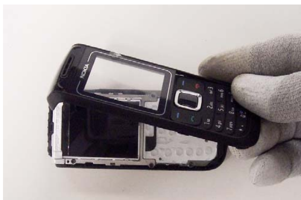
4) Lift and remove A-Cover and Keymat.
